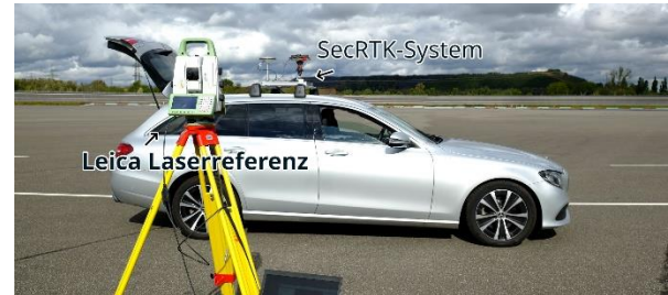
GNSS-independent reference system with Leica MultiStation
